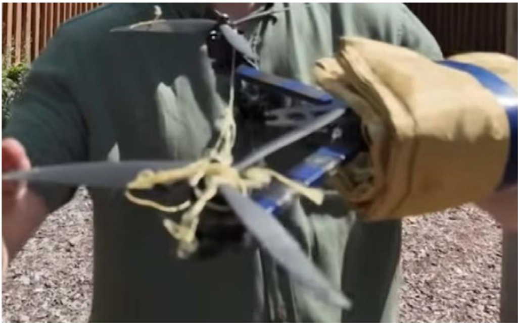
Photo 26. The result of defeating the drone with the "PEREKHVAT" bullet (Kevlar thread tangled the drone blades, 1 blade was cut off by the thread)
