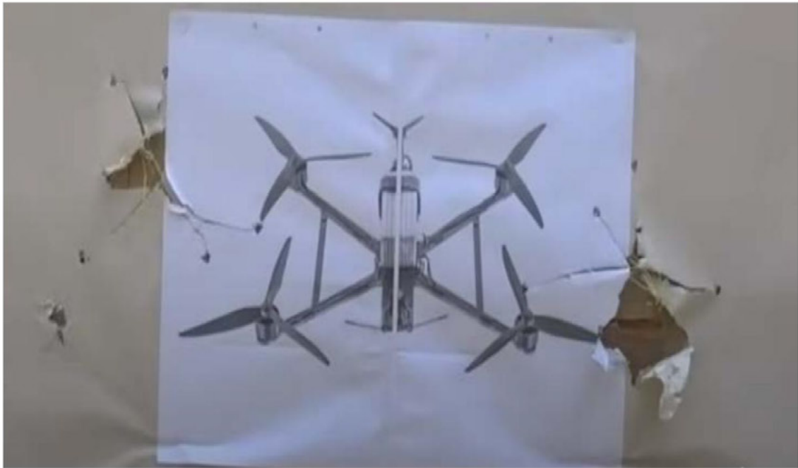
Photo 19. The testers fired 2 shots from a distance of 10 meters in order to show the diameter of the opening of the charge
