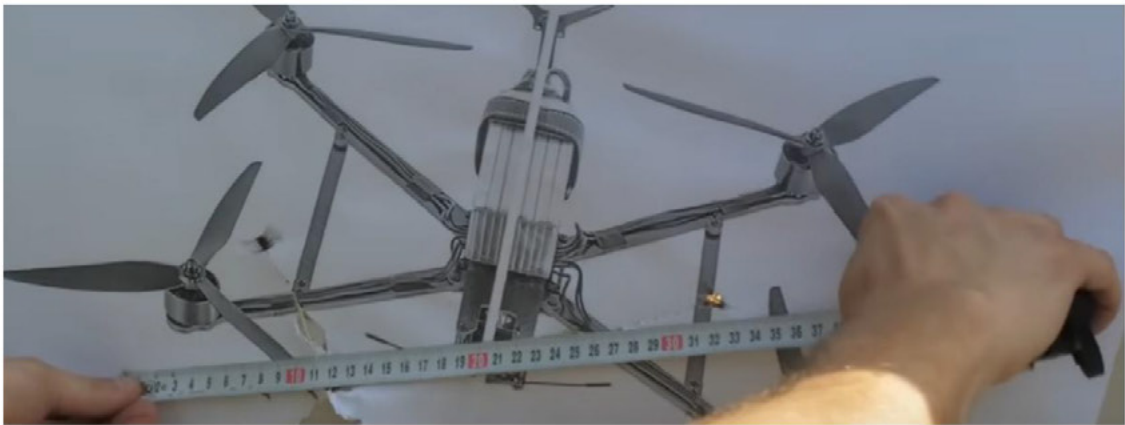
Photo 24. Showing the opening of striking elements at a distance of 30 meters (makes 33 centimeters)
